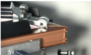
Rulmanlı kazıma sistemi Bearing scratching system
